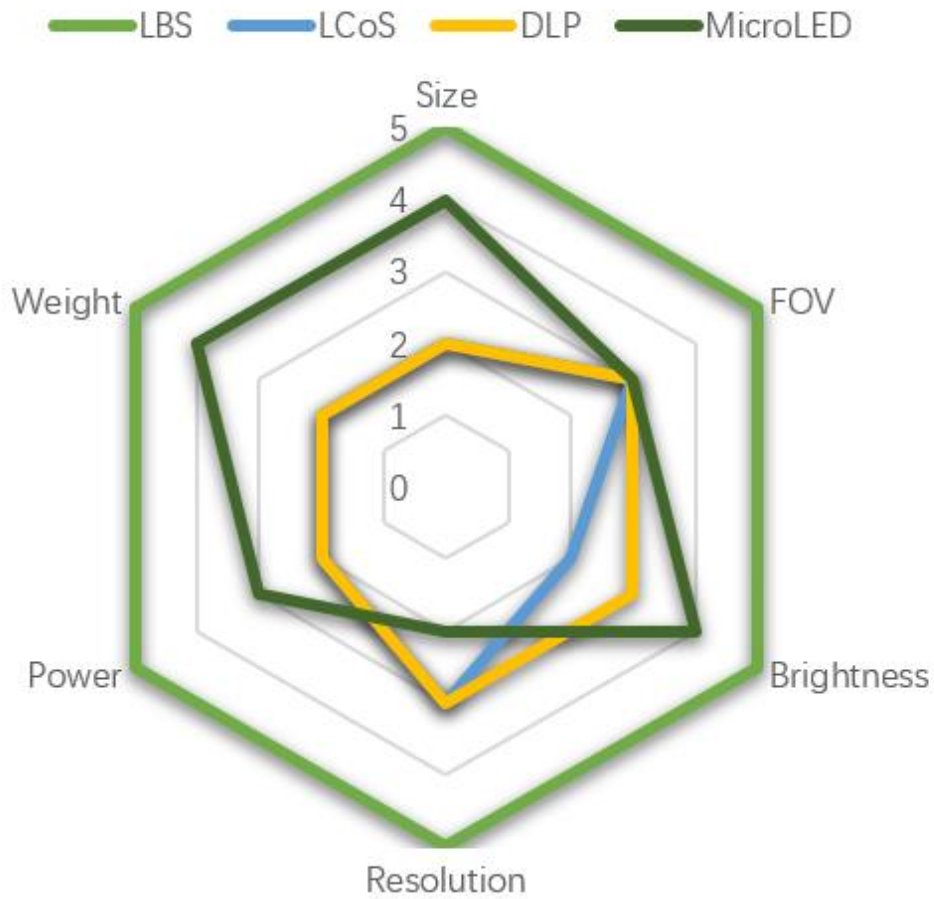
Figure 4: Comparison of important parameters among mainstream optical engines
